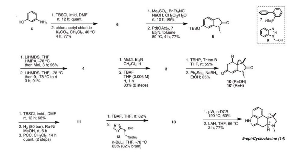
Part B: Second Generation Retrosynthetic Pathway: synthesis of (+-) Cycloclavine
