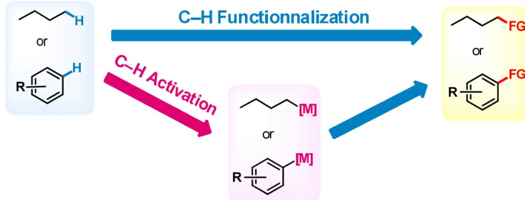
C-H activation: formation of a C-M bond with rupture of a C-H bond
